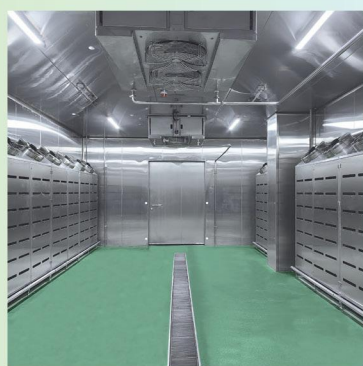
Air from the Side – Air Box Structure
